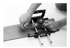
**Step 9** – Lock blade receiver (D) by pressing down the receiver latch lever (E).
