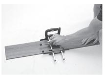
**Step 11** – Press firmly down on knob (A) and slide Ripper along the full length of your vinyl plank.
