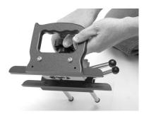
**Step 1** – Retract blade by turning depth knob (A) counterclockwise. You can stop when blade is fully retracted into the receiver. Continue to rotate knob if you would like to remove it completely.
