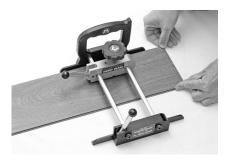
**Step 4** - Place the MARSHALLTOWN<sup>®</sup> Vinyl Ripper over a vinyl plank.
