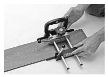
**Step 5** – Slide guide fence (B) up to the vinyl plank
