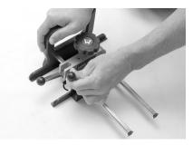
**Step 2** - Unlock guide fence (B) by lifting latch lever (C).
