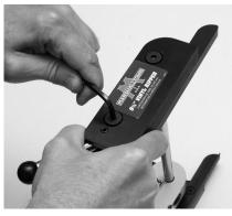
**Step 6** – Install and tighten Screws (F) into Guide Rods (D) using Hex Wrench (G).
