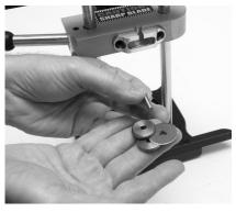
**Step 4** - Discard the old Blade and place a new one into the Axle Pin with a Spacer on either side of the Blade.
