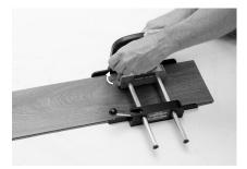
**Step 7** – Unlock blade receiver (D) by lifting latch lever (E).
