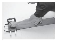
**Step 12** - Slide the Ripper off the end of the plank.
