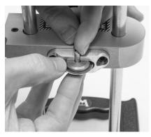
**Step 3** – Slide the Blade and Spacers out of the Blade Cartridge.
