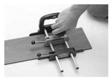
**Step 10** - Extend blade by turning knob (A) clockwise. Blade should cut into vinyl plank by about  $\frac{1}{1.6^{"}}$  (1.5mm).
